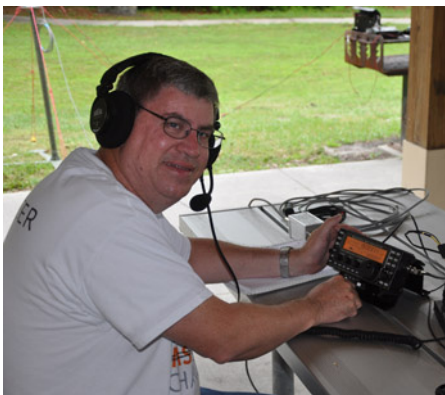
Dave, KU0R running CW on a new Elecraft KX3 at 5 watts into hamsticks on 17 meters at 20 feet. The power source was a LiFePO4 rechargeable 9 Ahr battery pack.
