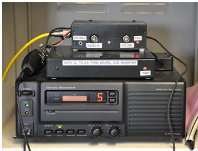
A close up view of the business end of the IRARC 145.37 MHz repeater (Yaesu Vertex 7000) and controller hardware located at Broadcast Court in Cocoa.
